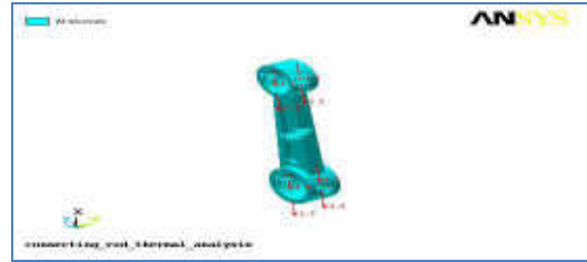
Fig. 5. Loads and Boundary Conditions
